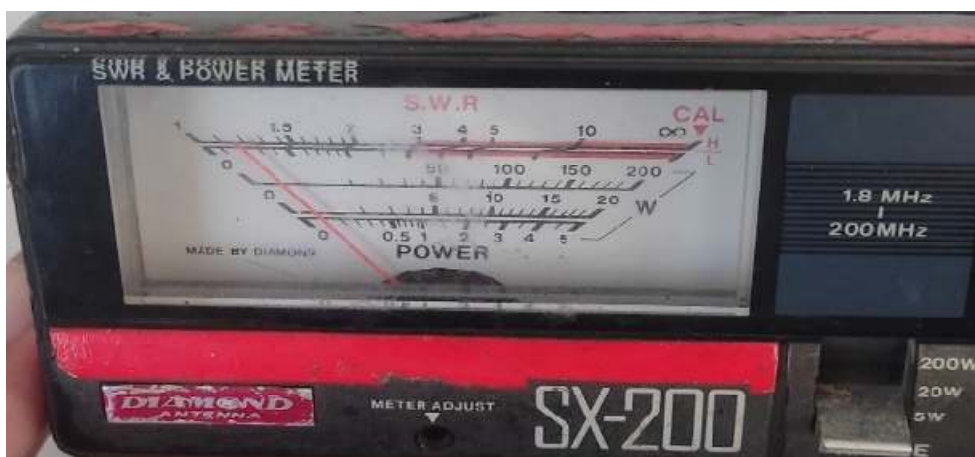
Gambar 3. Nilai vswr antena Telex
