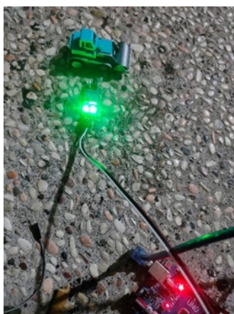
Gambar 12. Pengujian Sensor Infrared Terhalang Objek
